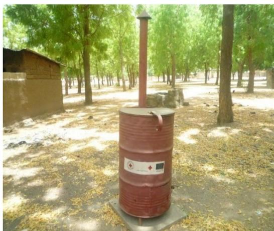
**Figure 6:** Local incinerator for Syringes
