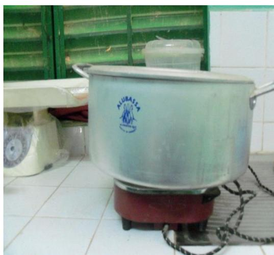
Figure 10: Disinfection of sharp materials in pots by boiling on heating plate
